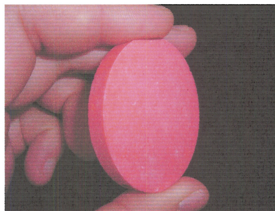
Fig. 3 Pressed cyanuric acid pellet.
